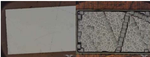
Fig. 4: Choline hydroxide etching progress at t=0min (left) and t=40min (right). Optical views at 2.5X.
